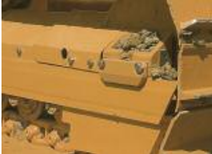
Smooth, tapered track covers provide easy undercarriage cleaning.
